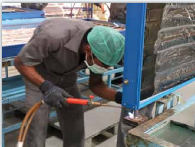
Collector Flange Brazing
