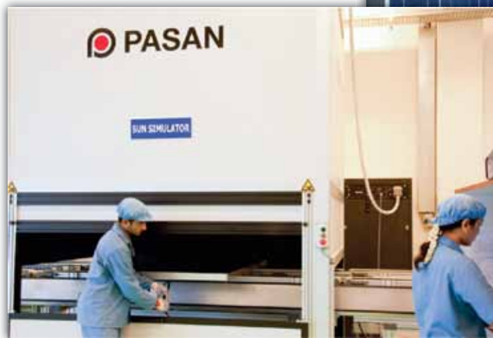
PASAN-flash generator-sun simulator of performance class A for measuring the output under standard test conditions at EMMVEE production facilities in Bengaluru, India
