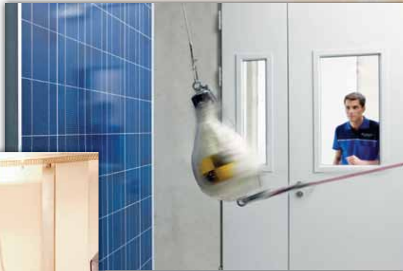
Module breakage test at the testing laboratory TÜV Rheinland in Cologne (Source: TÜV Rheinland)
