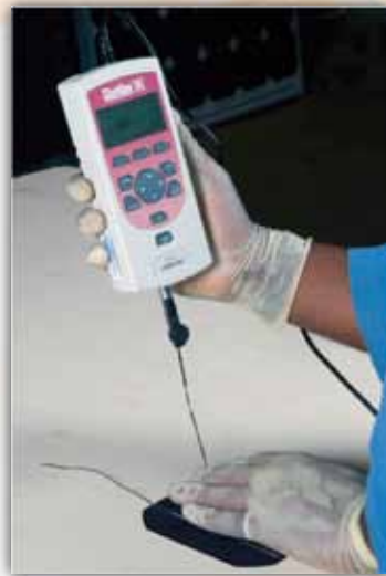
Pull test for the cell and string connectors during quality control at EMMVEE production facilities in Bengaluru, India
